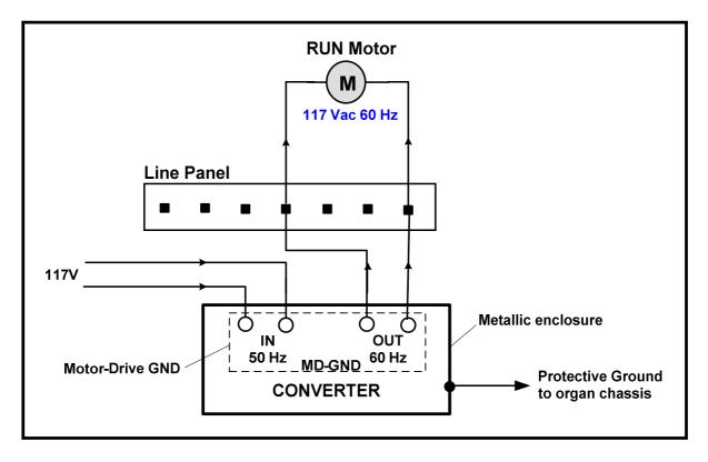
The converter should be installed on the left side of the organ (rear side view) preferably nearby the line panel aside the RUN motor.
