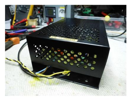
The first reason of installing this 60Hz PCB in a metallic enclosure is firstly to protect the user again electrical shocks since the entire PCB is connected directly on the AC Mains network. Another purpose of having this enclosure is to minimize EMI, if any (Electro Magnetic Interferences).
