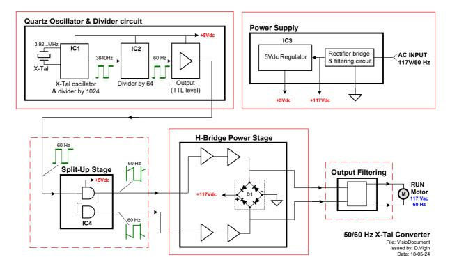
A shown on the block diagram, this 60Hz converter is composed of several sections:
