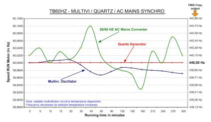
On the graph here-above, one can see the various fluctuations of the A-440Hz in function of the driven frequency. The X-Tal (quartz) solution provides the perfect stability while the two others may become 'out of tune'.
