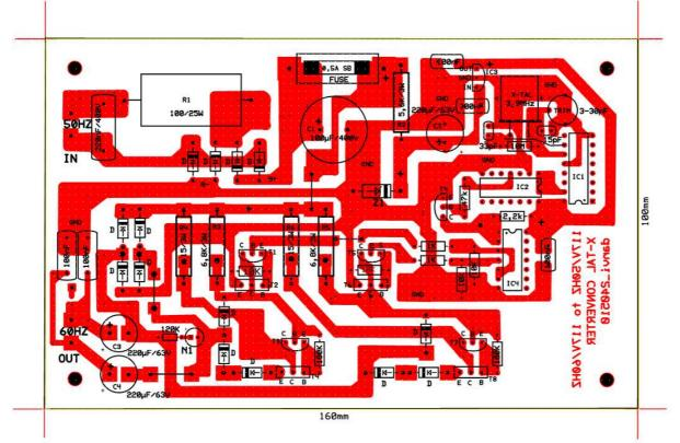
As already mentioned, there are no galvanic connections between the PCB and the metal enclosure. The fixation holes on each corner do have sufficient clearance to meet the European safety regulations.
